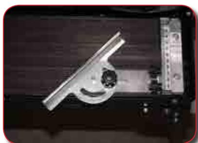
PROTRACTOR FOR CROSS CUTTING ANGLE
